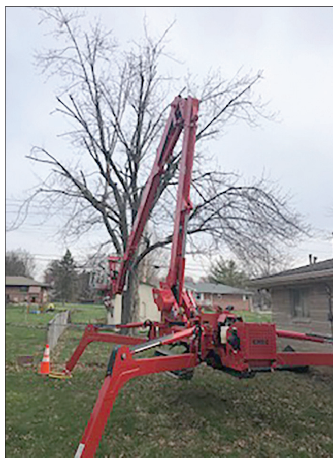
SUBMITTED PHOTO Paul Morton, who owns Airborne Tree Service, has an 83-foot boom that can fit through a 42-inch gate when its legs are contracted.
