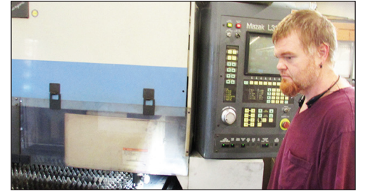
Sixth-year employee Mike Pope checks quality of small parts being stamped by the CNC Super Turbo Laser to be used with the Perfect Swing.
